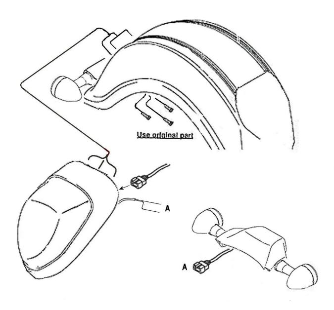
A: Turnsignal Left: Blue wire connect to OEM wire Turnsignal RightYellow wire connect to OEM wire
